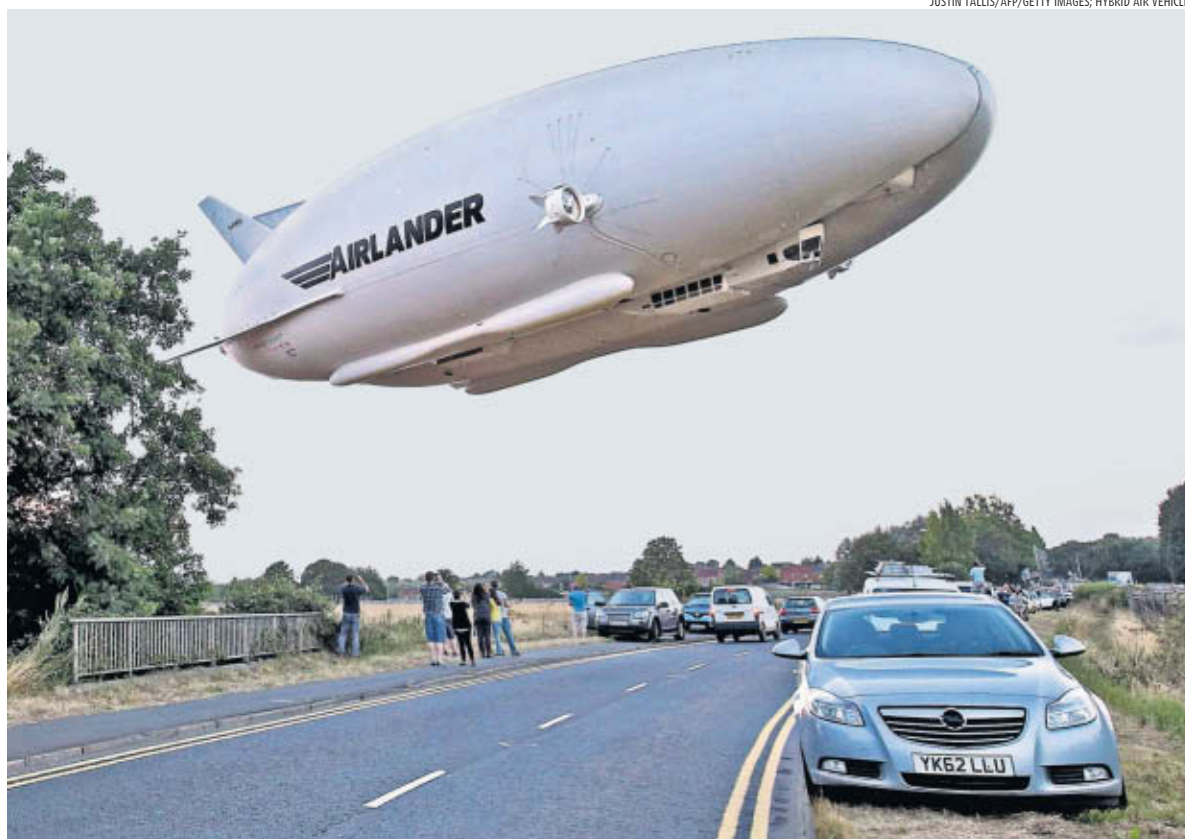
The Airlander stops traffic during a trial. It could have more than a hundred seats and is capable of carrying ten tonnes
